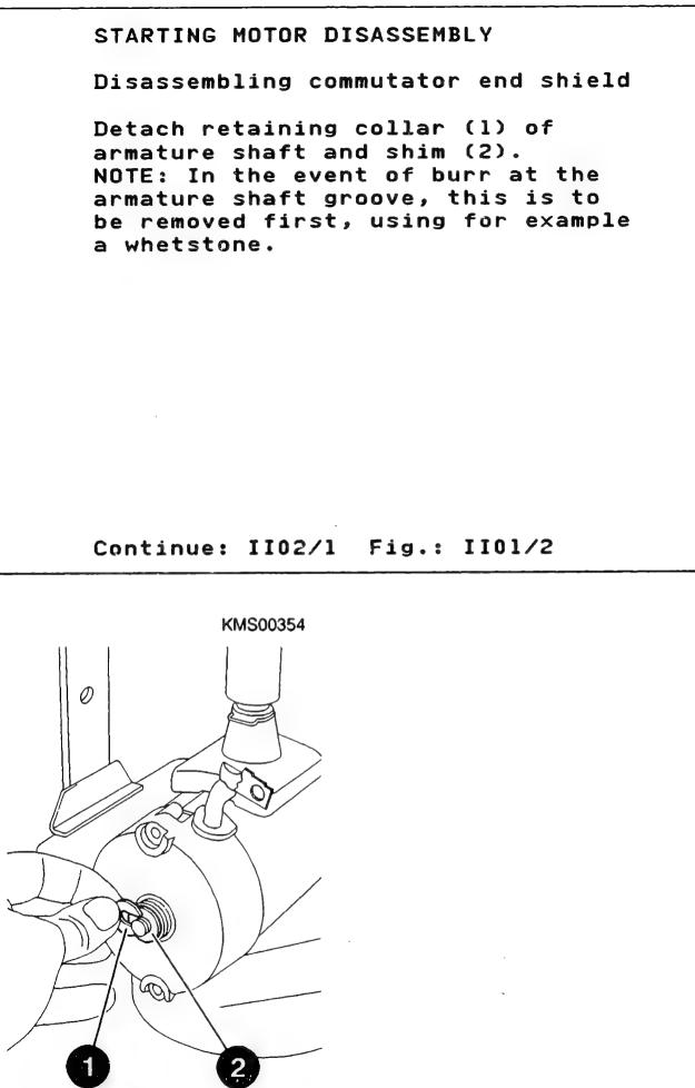
Disassembling commutator end shield
